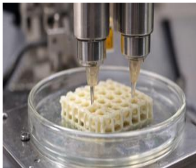
Fig. 3. Extrusion-based 3D bioprinted scaffold
