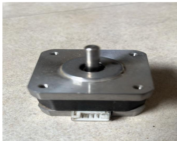
Fig. 2. Highly critical actuation subsystems: NEMA 17 Stepper Motor for high torque and accurate positioning, and All, metal Hotend assembly with a ceramic heating cartridge for stable thermal regulation.
