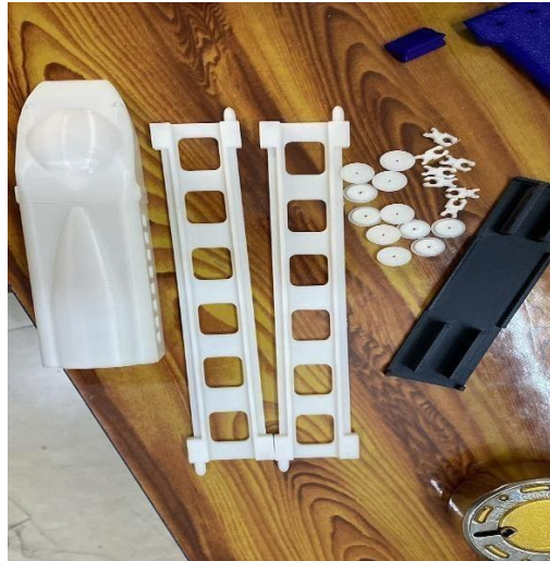
Fig. 3. Manufacture of a complicated multi, component railway assembly. The demonstration of the system's precision in measurements by the successful mating of wheels, axles, and chassis slots is less than 0. 2mm.
