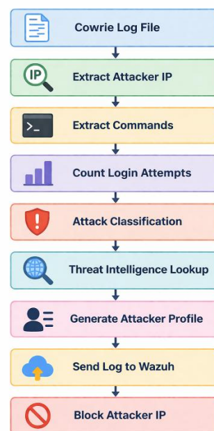
Fig. 4. Attack lifecycle and defensive workflow depicting the sequence from initial network scanning and brute-force attempts through honeypot interaction, command logging, AbuseIPDB threat intelligence verification, and automated firewall-based IP blocking
